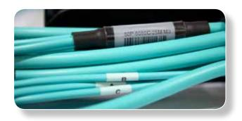
The Slack ZERO™ trunk cables are labeled to identify the Rack #, U #, and Port # of both the access and infrastructure racks. The labels appear every 2 feet to help facilitate installation and maintenance.
